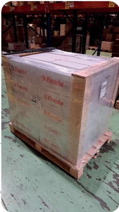
Wooden frames used to protect pallets in transportation
